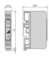
Fig. 10. SINEAX TI 816 on top-hat rail EN 50 022 –  $35 \times 7.5$ .
