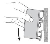
Fig. 3. Mounting onto the G-type rail.
